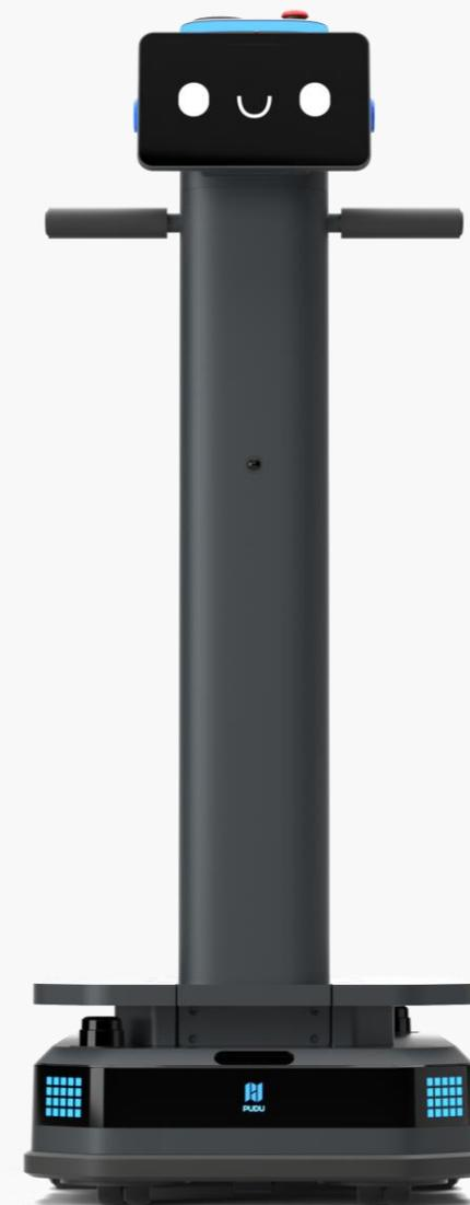
\*The T300 with lifting functionality will weigh approximately 80kg.
